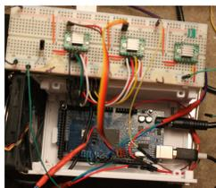
Figure 11: Stepper drivers and Arduino
