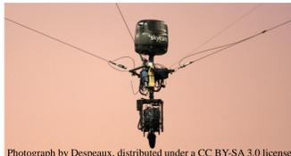
Figure 3: Skycam camera system.
