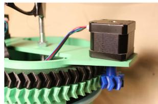
Figure 10: Pan tilt stepper motor
