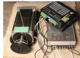
Figure 7: Stepper motor, driver, and PSU
