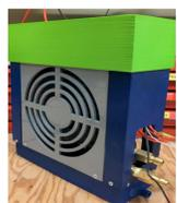
A breathable fabric cover allows for easy mounting. The internal skeleton is made of PLA.
