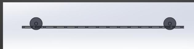
Solution is to attach **two dead axles** to the system and then add **wheels and bearings** on the ends of the axles, so it can be easily pulled out with a **winch**.
